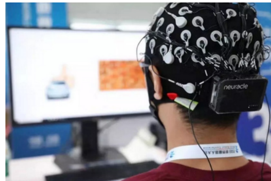
Figure 2.17 Non-invasive AAC-BCI setup, a user wearing an EEG cap connected to a communication interface on a computer screen (Brain-Computer Interface (BCI) Explained - RoboticsBiz, 2021)
