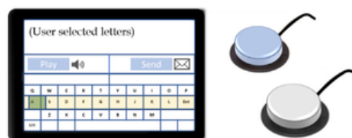
Figure 2.11 A sample visual scanning interface activated via switch scanning using the buttons (Elsahar et al., 2019)
