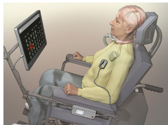
Figure 2.18 Implanted BCI spelling system enabling communication via a brain-computer interface, with an on-screen letter grid controlled through neural signals (Brain-Computer Interface in a Locked-In Patient | NEJM, 2016)
