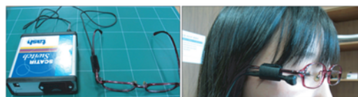
Figure 2.10 Self-Calibrating Auditory Tone Infrared switch (Park et al., 2012)
